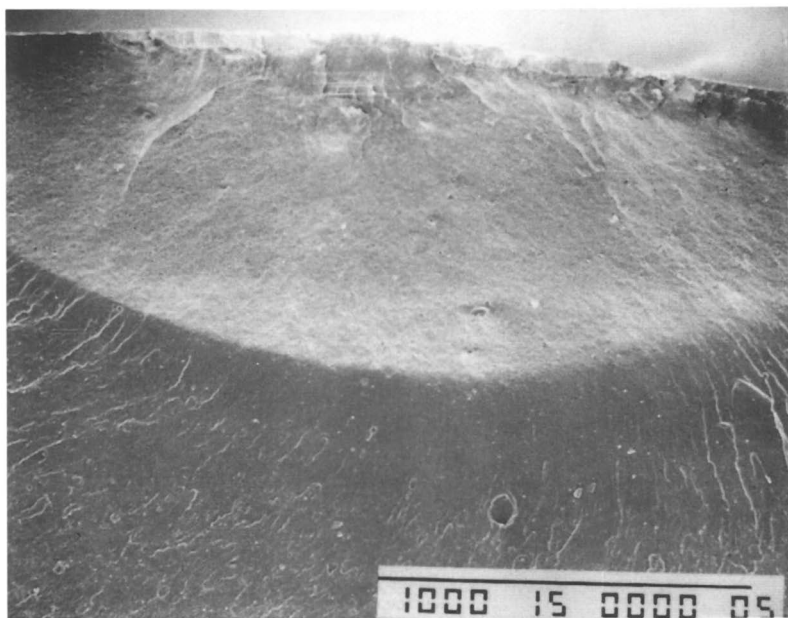
Figure 18. SEM Image of Fracture Point of a Vulcanized Natural Rubber Specimen after Four Months of QUV Exposure. (50X Magnification).
