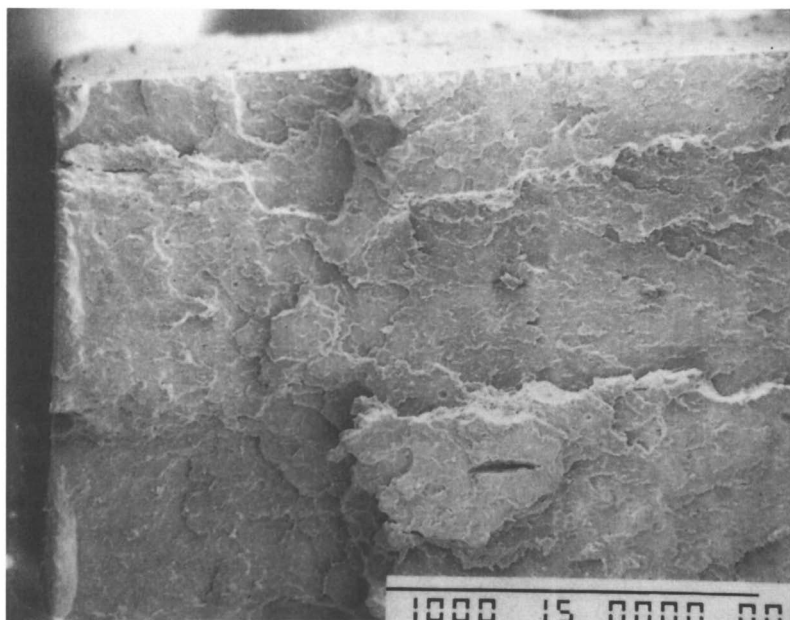
Figure 16. SEM Image of Fracture Point of an Unexposed Vulcanized Natural Rubber Specimen. (50X Magnification).
